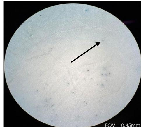
**Figure 11: Analysis of a 1:100 test sample using 4x magnification (arrow highlighting agglutination)**
