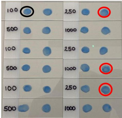
Figure 4: A photograph of completed LAAs on microscope slides using all the designated  $A_G$  concentrations (circled in black is the control test and circled in red is the live  $A_G$  test)
