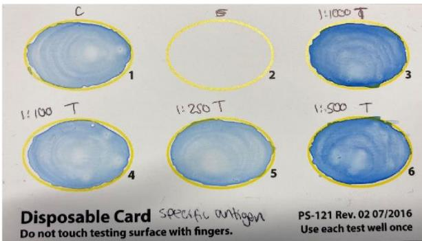
**Figure 8: LAA completed on a specialised disc card for all A<sub>G</sub> concentrations**
