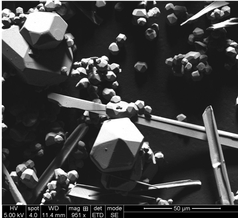
Figure 9: Pyromorphite heated to 900°C with 5 hour isotherm
