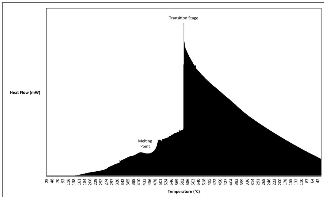
The main use of the TGA was to heat small samples to different temperatures to determine whether crystals would form from a melt and, thus, which temperature gave the best crystals of pyromorphite. Samples of pyromorphite were heated over a range of temperatures, reaching the maximum of the machine at 1000°C. The XRD spectra patterns were then taken for each temperature reached, and compared to each other. The spectra are shown in Figure 3.
