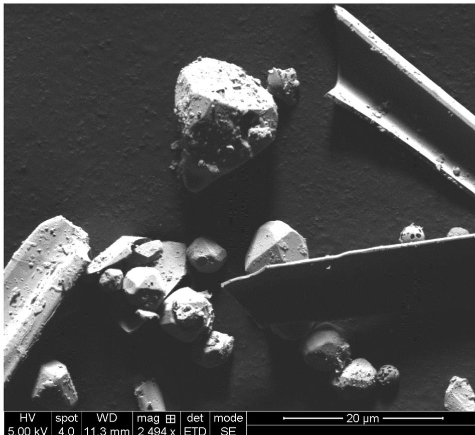
Figure 8: Pyromorphite heated to 700°C with 5 hour isotherm
