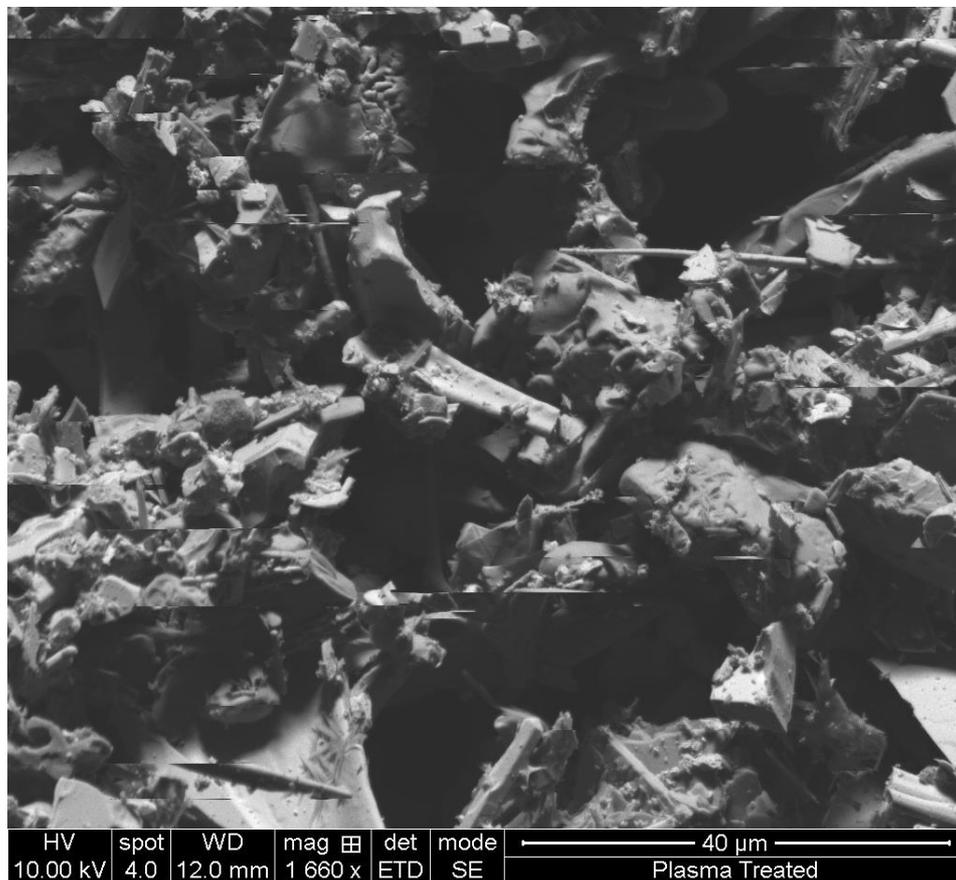
Figure 10: Pyromorphite heated to 700°C with 5 hour isotherm followed by 50-hour cooling step
