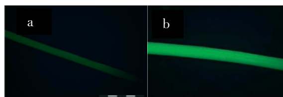
Figure 3: Comparison of fluorescence in two strands of hair which have undergone different levels of oxidation. (a) Untreated reddish-blonde (b) hydrogen peroxide treated dark blonde hair.
