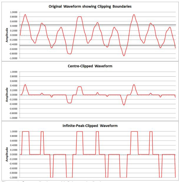
Figure 4: Centre-clipping and infinite-peak-clipping
